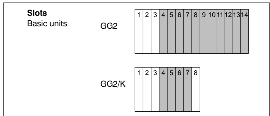
Fig. 5-2 System modules, slots
